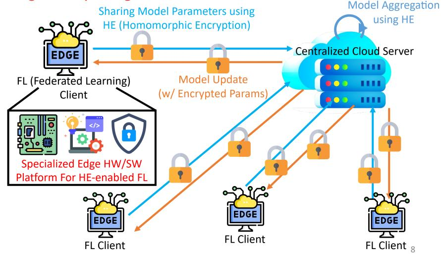
Target System for Platform Design: FL client w/ HE running on the edge
