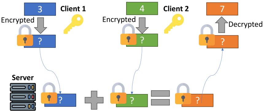
Arithmetic computation over ciphertext (encrypted data) w/o knowing crypto key or plaintext (unencrypted data)
